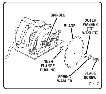
**NOTE:** The saw teeth point upward at the front of the saw as shown.
